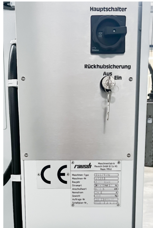
Detail view of machine rear side with main switch and nameplate
