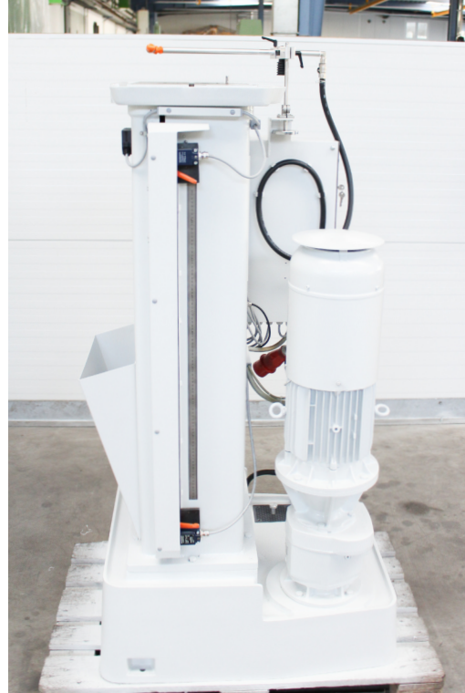
View of right side of machine with external adjustment of clearing stroke
